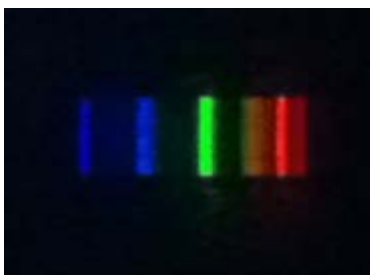
FIG. 6: Compact fluorescent light spectroscope image; courtesy Klaus Woelk, Missouri S&T
