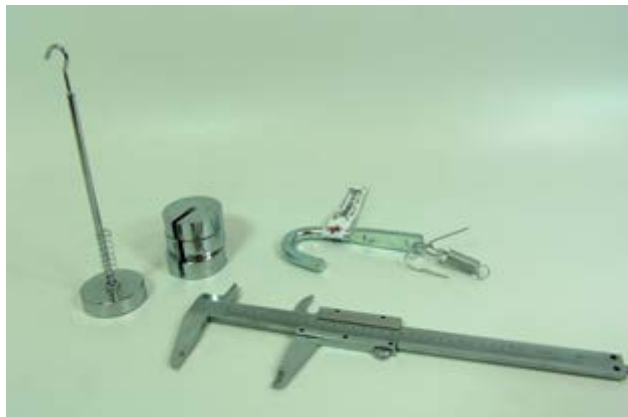
FIG. 1: Mechanics of materials spring constants and linear regression kit components; photo courtesy Jeff Thomas, Missouri S&T
